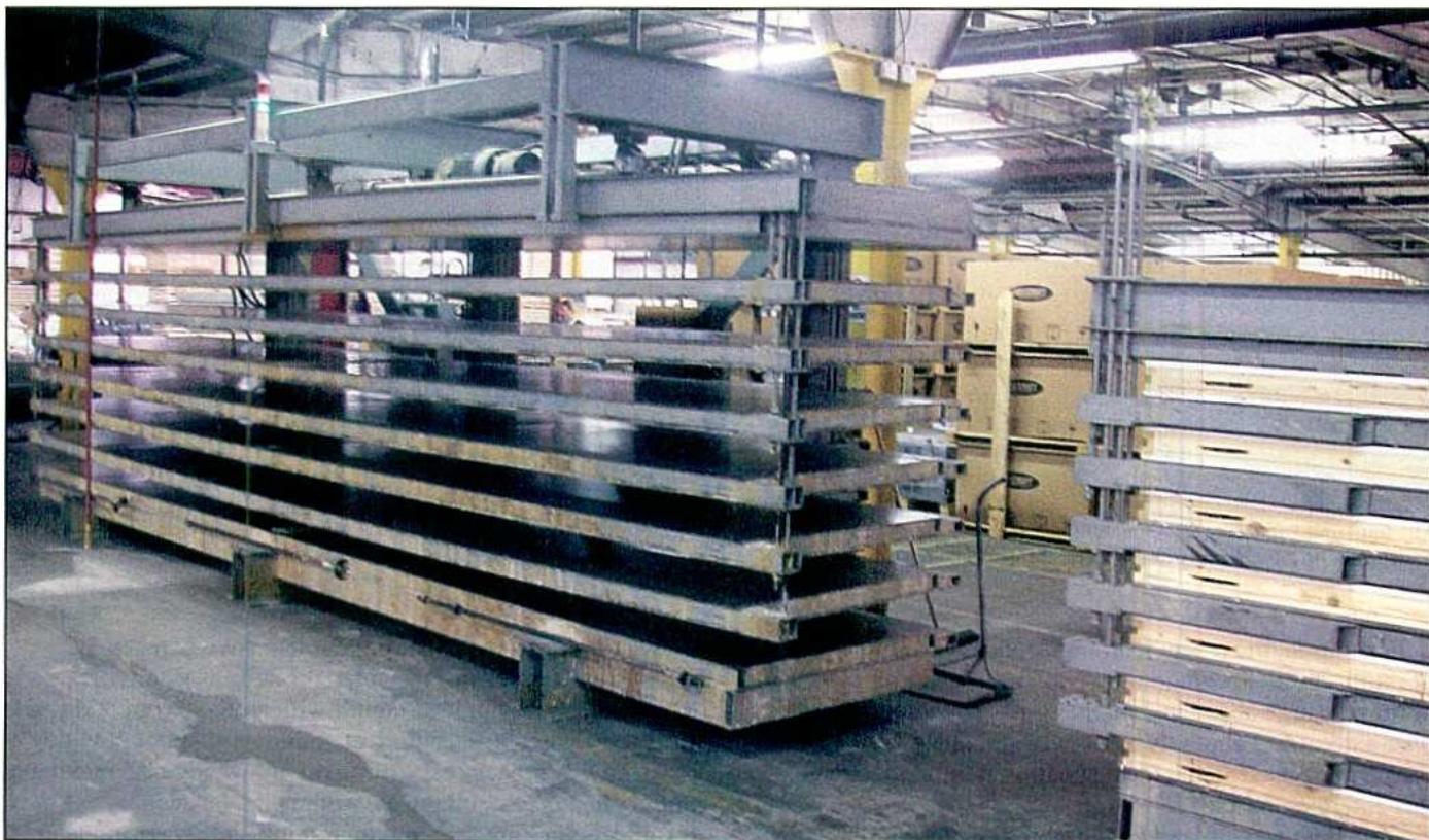
The high production facility in Atlanta, GA uses custom made seven-tier presses and each press has the capacity to produce 24 polyurethane panels per hour.
