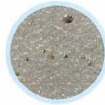
HFC-134a Somewhat uneven densities Somewhat weak adhesion Small voids in foam
