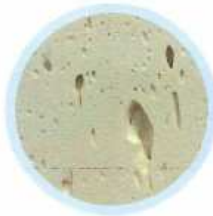
HCFC-22 "Tear Drop" Voids in foam Somewhat uneven densities Good adhesion to skin
